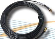
**RG-174** is a very small (approx. 0.1"/2.5 mm) flexible cable best suited for mobile/portable applications up to 1900 MHz. It can be used in short runs up to 2.7 GHz. For miniature sized connectors it has the widest options available.
