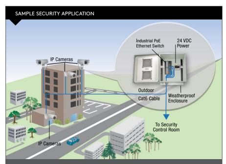
This sample security application illustrates the use of outdoor NEMA enclosures for video surveillance on a typical building. L-com includes NEMA enclosures with industrial PoE switch, 24 VDC power, outdoor Cat6 cable and IP cameras.
