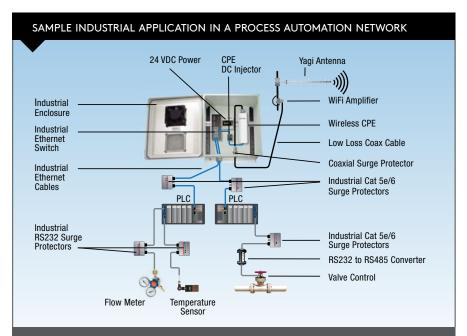
This diagram encompasses a rugged indoor NEMA enclosure, along with Ethernet, RS232, RS485 and WiFi connectivity, to provide an end-to-end process automation networking solution.
